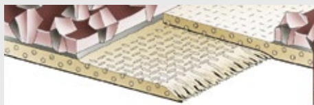
Typ 2: Overlapped joint with grit sanding
