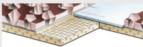
Typ 4: Butted joint with special film on the grit side
