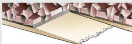
Typ 1: Overlapped joint without grit sanding
